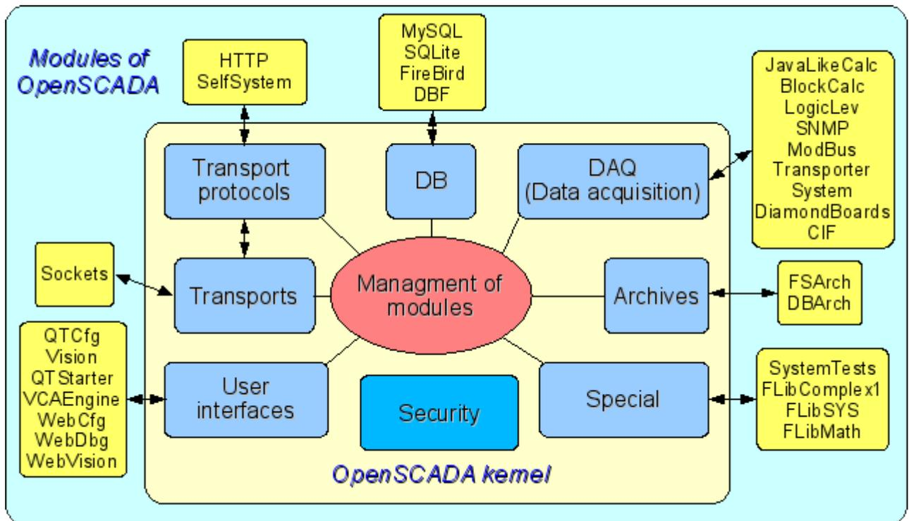
Рис. 1. The block scheme of OpenSCADA system
