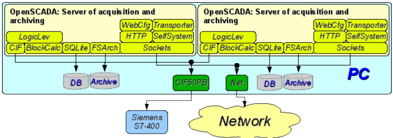
Рис. 5. The duplicated server connection on one server.
