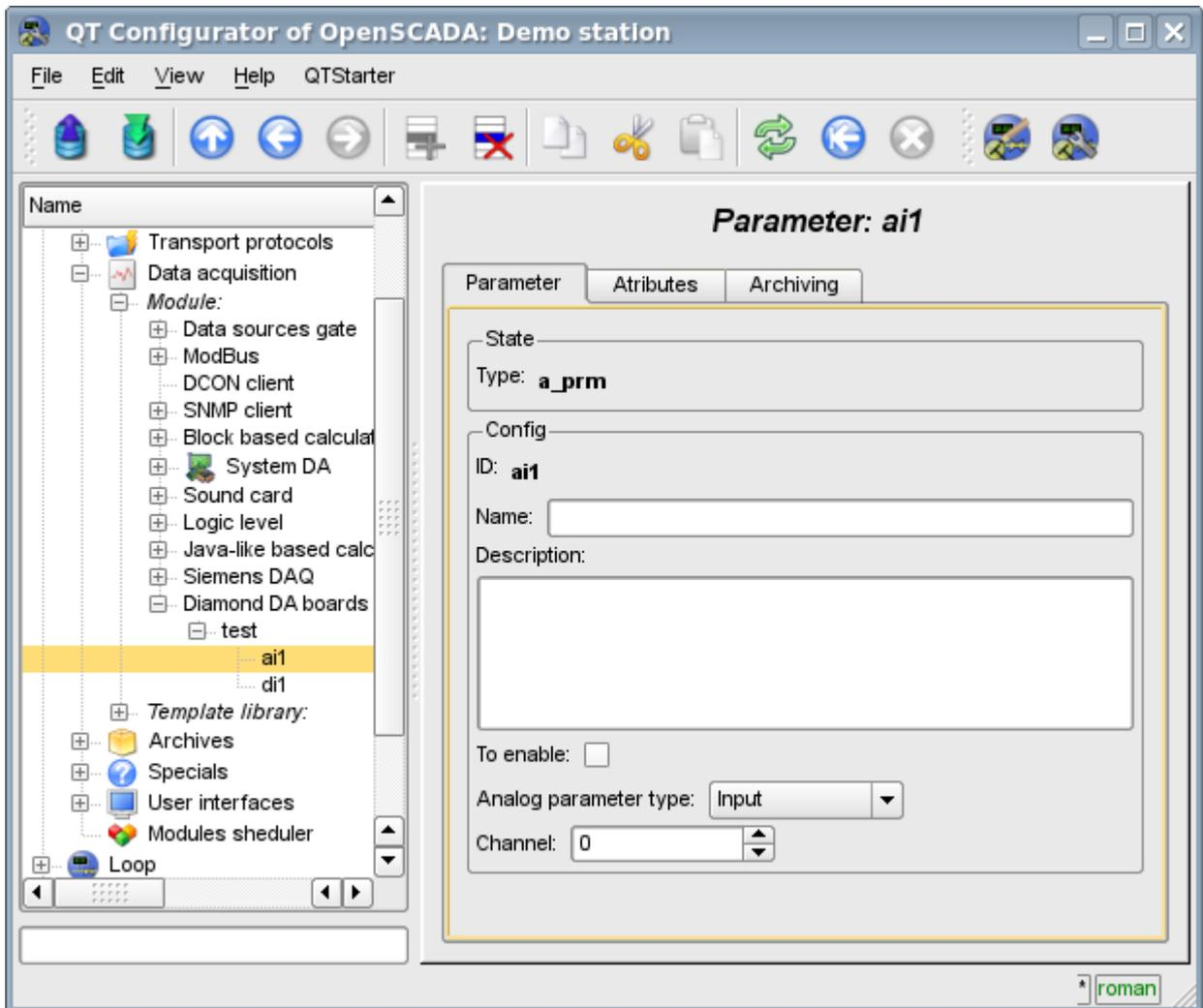
Fig.3. Tab of the configuration of analog parameters.
