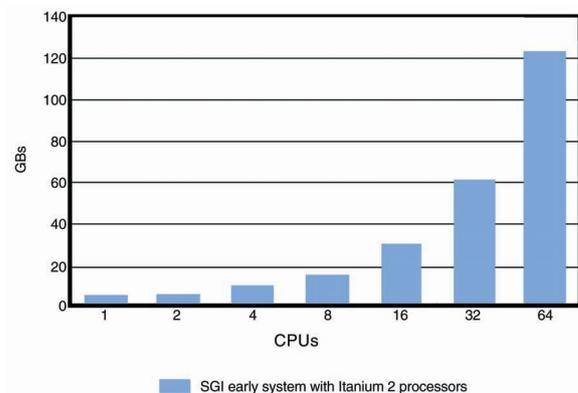
Figure 10. Near-linear STREAM Triad scalability up to 64 processors.
