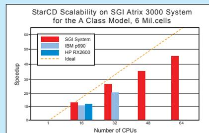
Figure III. STAR-CD results comparing Linux, HP-UX and AIX.
